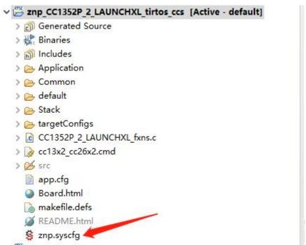
2. Enable serial flow control in the UART option in the .syscfg configuration file:
