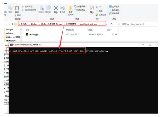
2) Enter the serial port number inserted into the dongle
