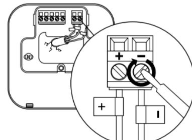
EN Common terminal labels on the boiler.
